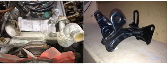
Further points of difference are the engine mounting brackets which are much larger on the Saloon and are not interchangeable with the Dart .
