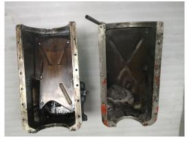
Note also how on the Saloon the oil filler tube is cranked to clear the air cleaner on Saloons fitted with the single, large air cleaner. The tube is straight on the Dart and on later Saloons where it is straight but a little longer. Any of the 3 can be used on a Dart and perversely, the increased length of both types of Saloon tube make for easier topping-up on a Dart!
