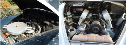
The most obvious difference on opening the bonnet is the carburettor air cleaner which on early models of the Saloon (left) is centrally mounted. Later Saloon versions had two smaller pancake filters (right) whereas Darts all have small, mesh-filled filters (below)
