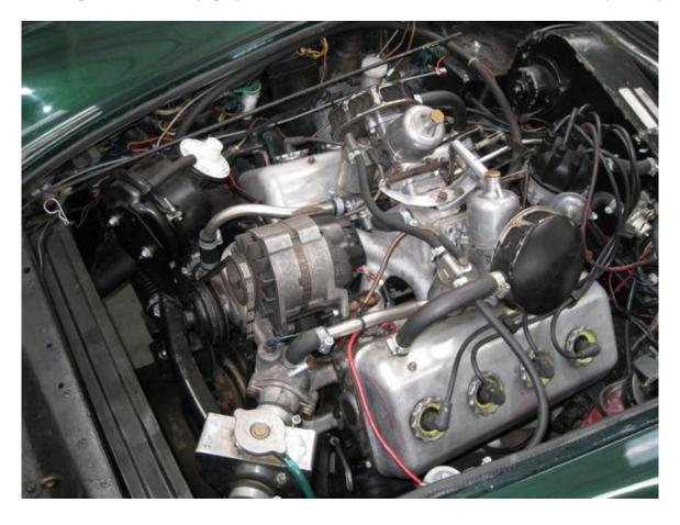
The Saloon distributor includes an electronic module to drive the tachometer (below,left) whereas the Dart has a cable drive.
