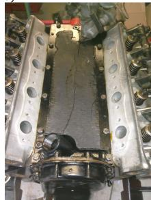
If you look closely at the two photographs of the oil reservoir beneath the camshaft location, you can see that the Dart engine (above, left) has two longitudinal webs either side of the cam bearing housings whereas the Saloon (above, right) has a single central web. This was presumably easier to cast and hence cheaper than the original Daimler treatment and can be found on very late Darts which used Saloon blocks.
