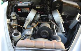
The most obvious difference on opening the bonnet is the carburettor air cleaner which on early models of the Saloon (left) is centrally mounted. Later Saloon versions had two smaller pancake filters (right) whereas Darts all have small, mesh-filled filters (below)
