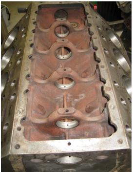
Moving on to the rear main bearing, you can see that the Dart unit (below, left) has an oil thrower arrangement while the Saloon is machined to incorporate a seal. Yes, the bearing shells are a touch worn!
